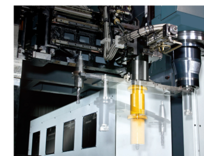
Extended head exchange on vertical type(opt.)
