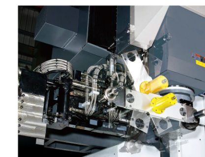
AC 90 degree angular head exchange on horizontal type(opt.)
